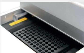
TE refrigeration using 72 long life series, the process in TE base plate and the semiconductor substrate using the new adhesive technology, make the TE also work normally under high humidity environment. and greatly improve the service life of the TE piece at the same time, through the experiment testing TE refrigerationservice life greatly increased.
